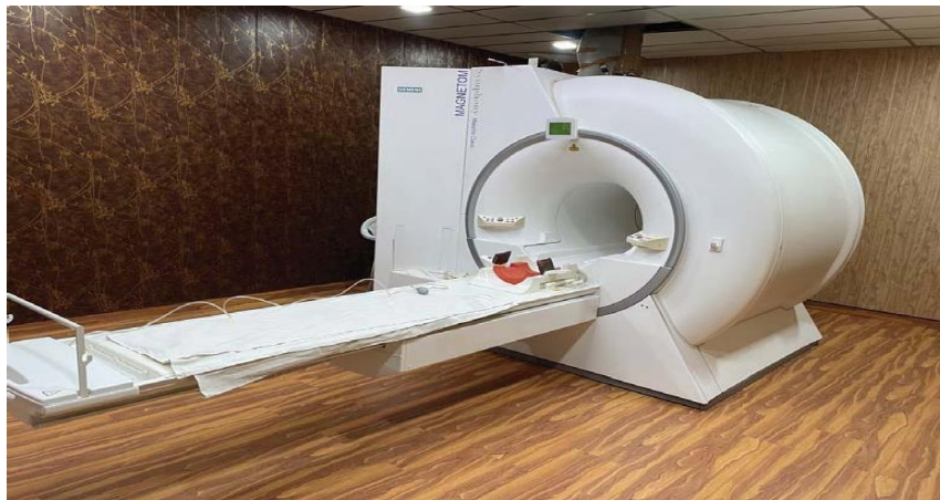
Fig.1- Siemens Magnetom Symphony 1.5 T, Quantum gradient and RF application system with Syngo windows based software version.
